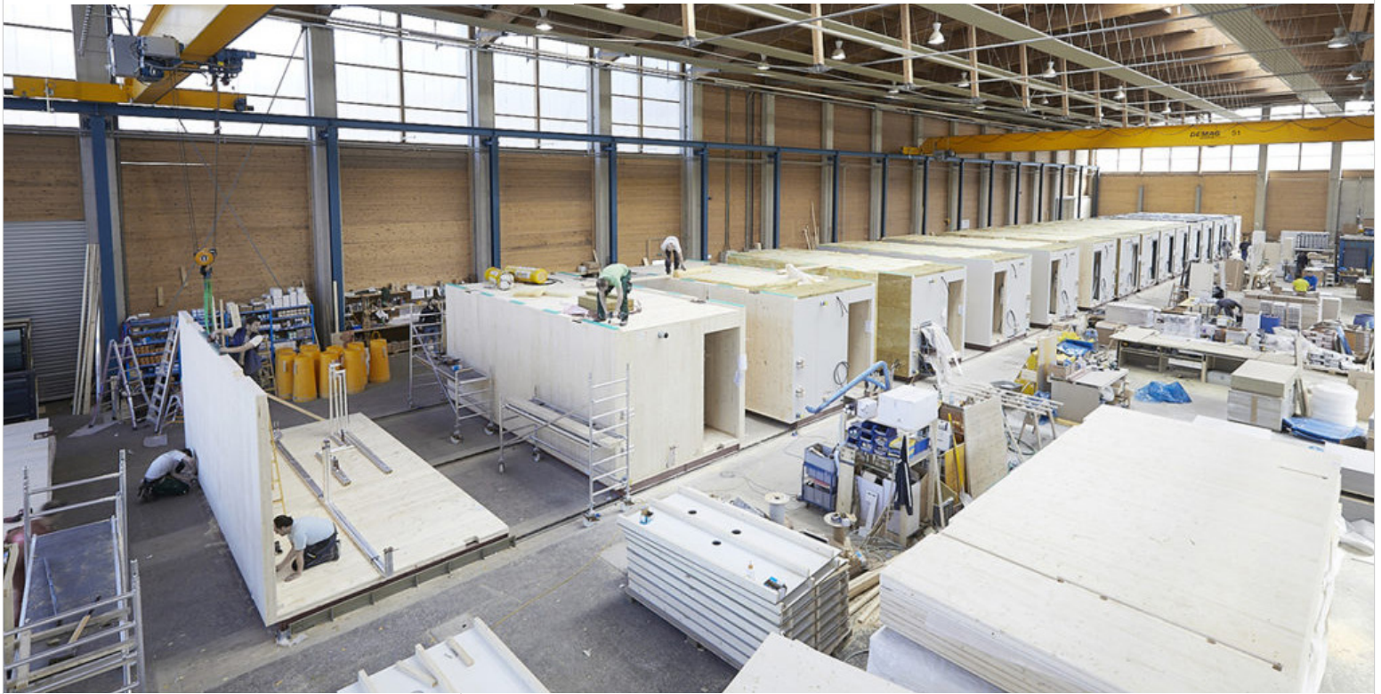
FIG 2: Kaufmann Bausysteme's 3D module production.
