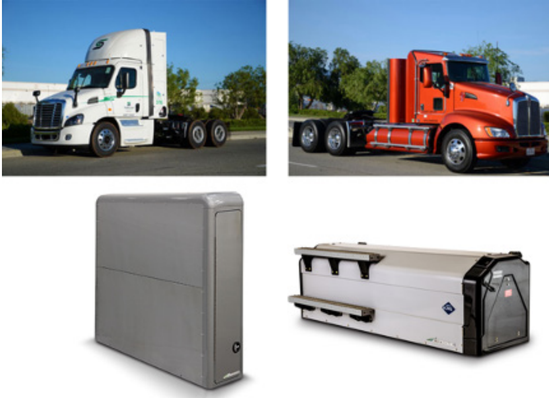
FIGURE 3.24 Behind the Cab and Side Mount Rail CNG Fuel Storage System
